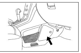
Pull the latch of the fuse box cover straight back to access the fuses.
